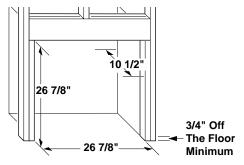
Figure 9 - Rough Opening for Installing in Wall
